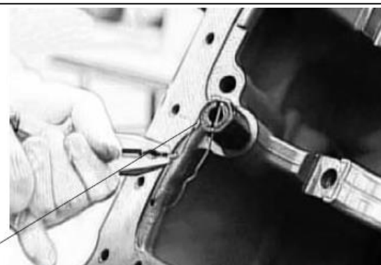
Fig 5-2 Pressure Limiting Valve of Oil Pump
