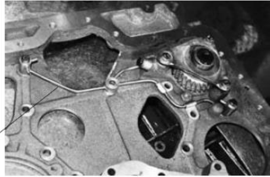
Fig 5-24 Lubricating Pipes Installation
