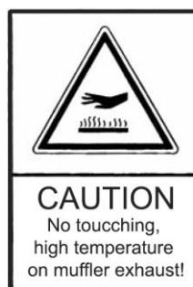
Fig.1-6 Located below Exhaust Pipe
