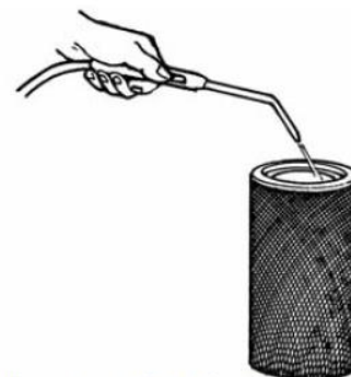
Fig 3-6 Clean Air Filter Element
