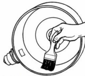
Fig 3-5 Clean Dust Accumulator
