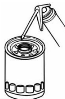
Fig3-12 Replace Oil Filter Element
