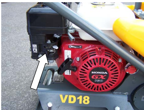
Fig. Closed fuel valve engine
