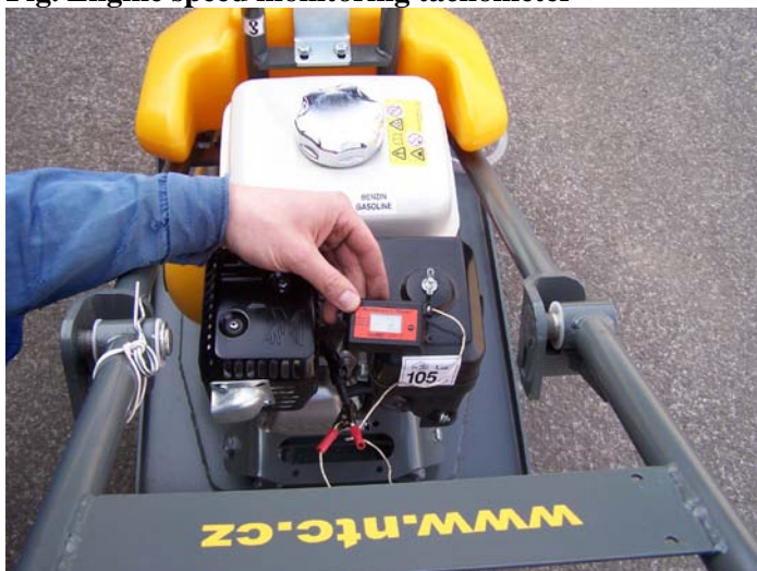
Fig. Engine speed monitoring tachometer
