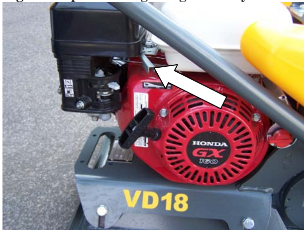
Fig. Lever position in gas engine slowly
