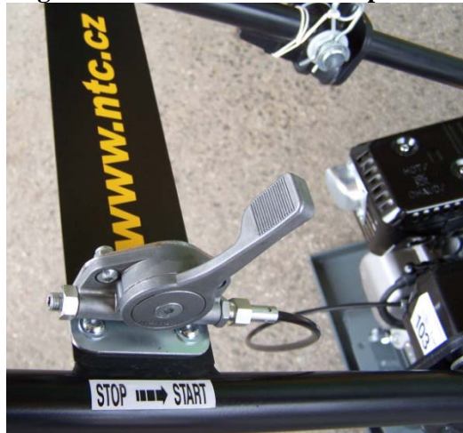
Fig. Throttle lever in the FULL position
