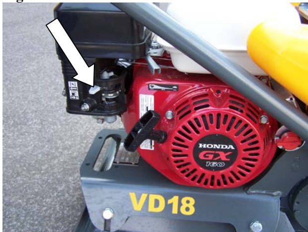
Fig. On the motor choke
