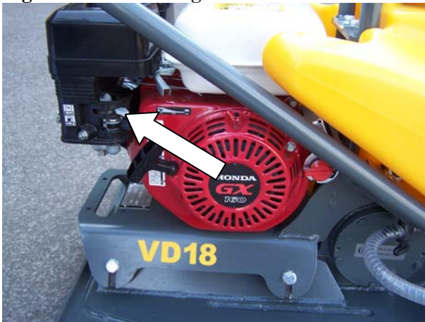
Fig. Choke off the engine
