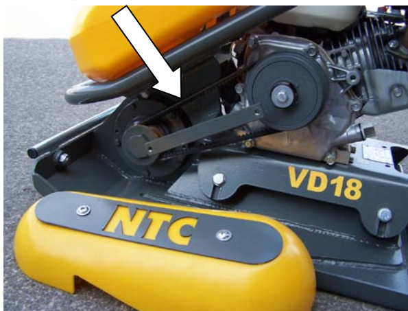
Fig. Inspection of drive belt tensioning
