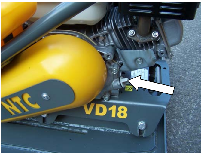
Fig. Check engine oil level
