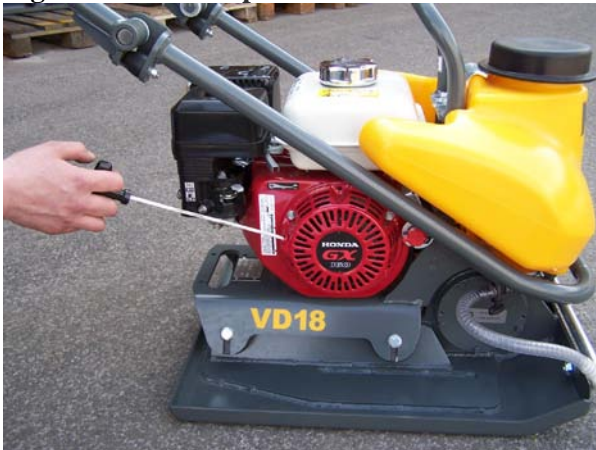
Fig. Starter motor pulled out cord
